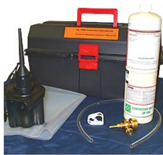
Figure one: Mercury thermometer, psychrometer and CO 2 sensor calibration kit at 1000 ± 20ppm.
